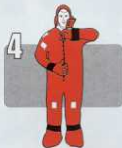
4 Insert other arm and close zipper and face flap. Adjust wrist and ankle bands to fit.
